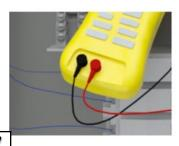
Press and hold the Current Clamp Trigger to open the red clamps.
