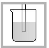
2. Laboratory test: Put the probe in a beaker that contains the solution. Do not let the probe touch the stir bar. bottom or sides of the container. Remove the air bubbles from under the probe tip. Stir the sample at a slow to moderate rate. Field test: Put the probe in the sample. Move the probe up and down to remove bubbles from the electrode. Make sure to put the temperature sensor fully in the sample.
