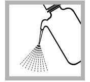
**1.** Rinse the probe with deionized water. Dry the probe with a lint-free cloth.
