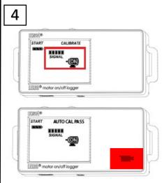
Press and hold the calibrate button until the screen displays AutoCalPass.
