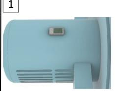
Place the motor on-off logger on the motor housing, use the magnets behind the logger to attach on the motor.
