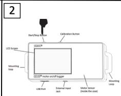
Press the start button on the logger to initiate the logger.
