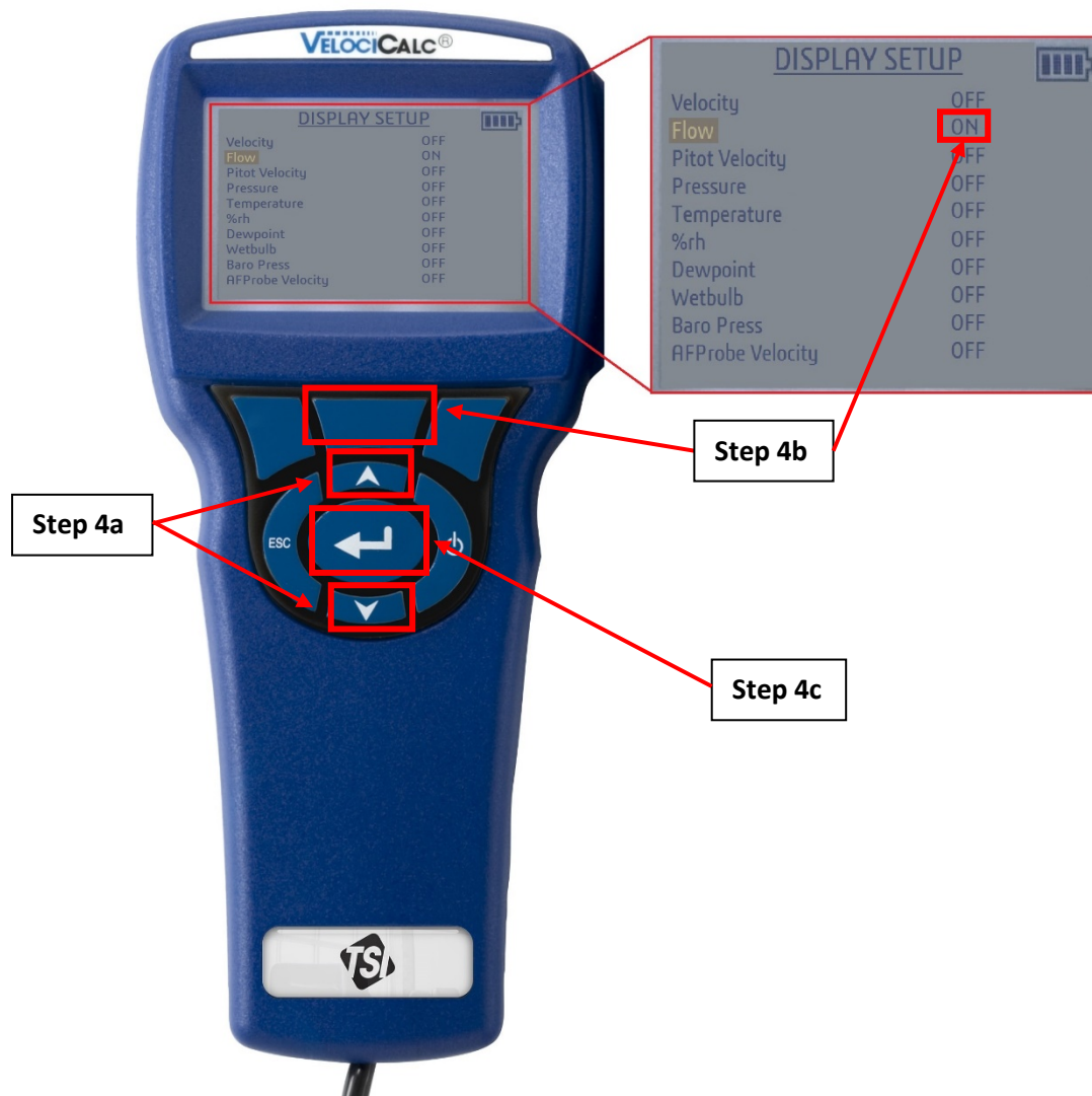
Figure A.10.2: The “Display Setup” screen for the TSI-9545 Air Velocity Meter. As an example, “Flow” has been set to “ON”. The instantaneous flow measurements in CFM that are being picked up by the meter will be displayed on the screen once the initial setup is complete. Since all the other options are set to “OFF”, only the flow measurements will be displayed on the screen.
