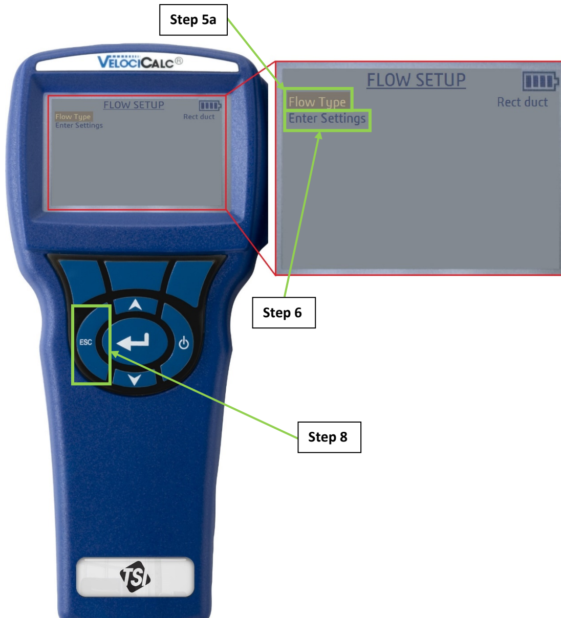
Figure A.10.3: The “Flow Setup” screen for the TSI-9545 Air Velocity Meter
