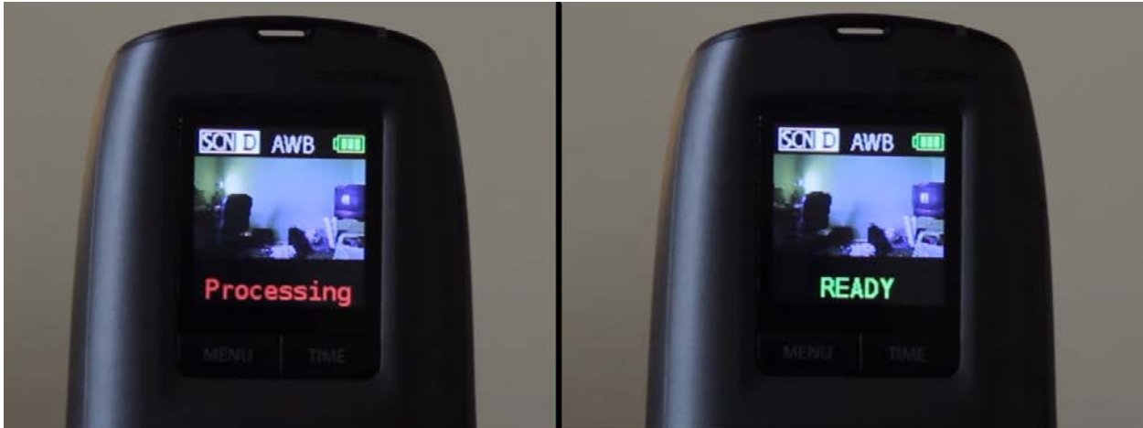
Figure A.11.14: The preview screen will display the word “Processing” as shown on the left which means that all of the time lapse photos are being processed into a .AVI video. Then the word “READY” will be displayed on screen as shown on the right which means that the SD card can be extracted, or a new set of time lapse photos are ready to be recorded.
