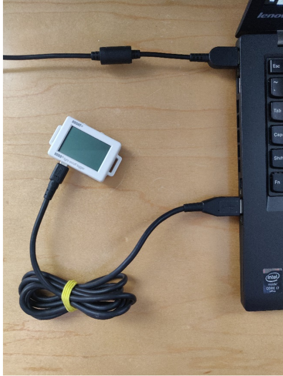
Figure A.9.1: Onset HOBO 4-Channel Analog Logger connected to computer via USB.
