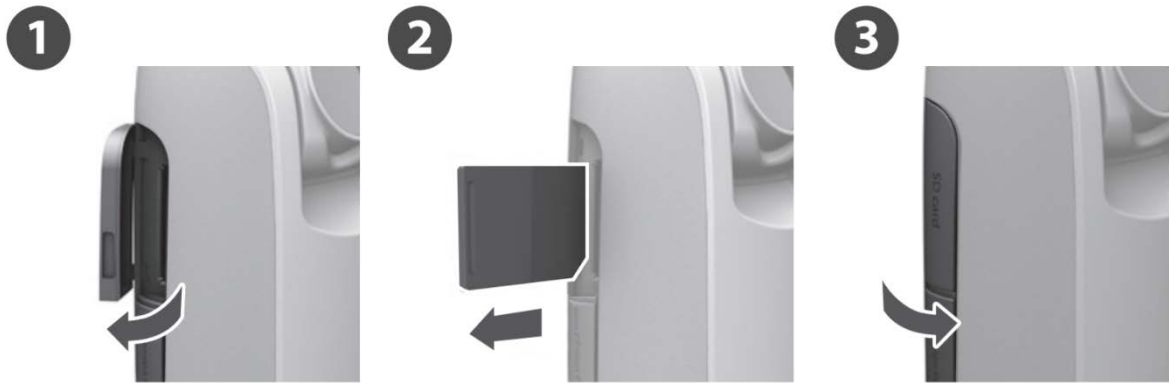
Figure A.11.15: Open the SD card cover as shown on the left. Extract the SD card as shown on the middle. Close the SD card cover in order to prevent dust and debris from entering the Brinno TLC200 Pro Time Lapse Camera as shown on the right.
