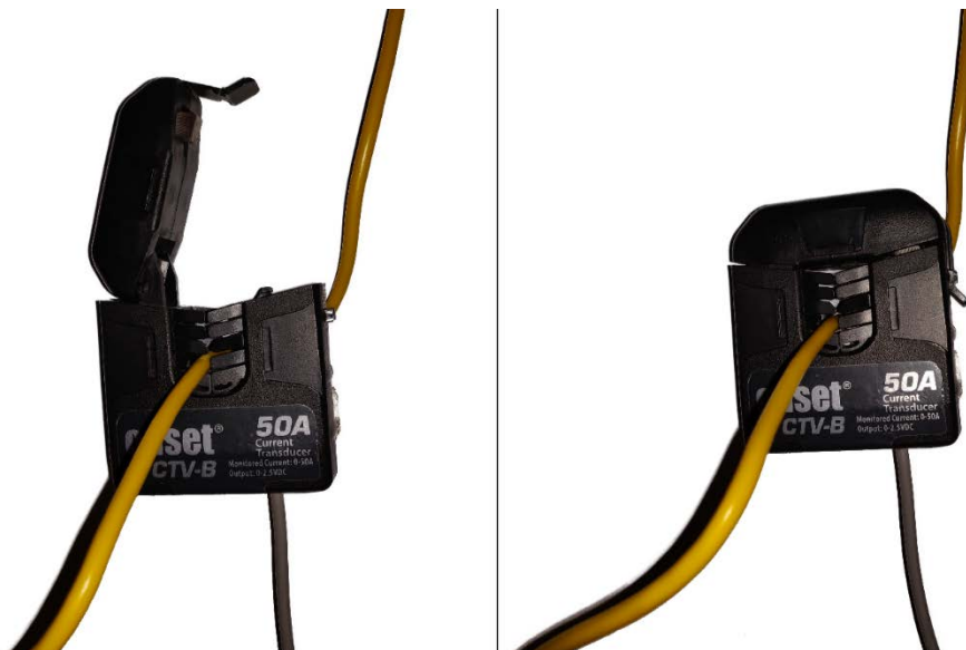
Figure A.4.11: Insertion of wire into the Onset HOB0 Split-core AC Current Transformer.
