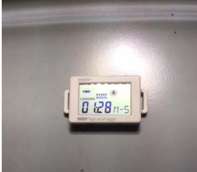
Figure A.5.8: Onset HOBO Light On/Off Data Logger attached to metal surface.
