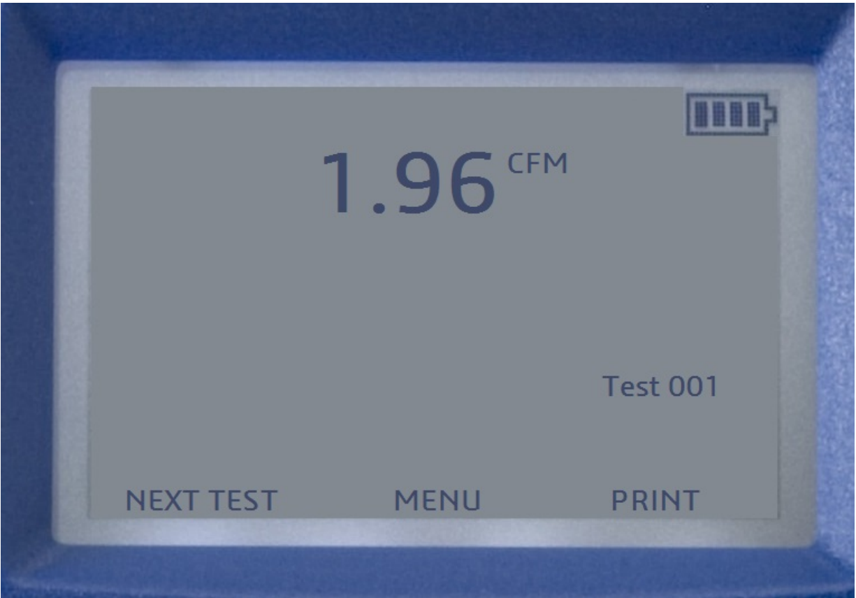
Figure A.10.10: An example screenshot of the TSI 9545 Velocicalc Air Velocity Meter screen after the initial setup is complete. Notice that only the flow measurements in CFM are displayed on the screen as a result of “Flow” being the only parameter selected on Figure A.10.2.
