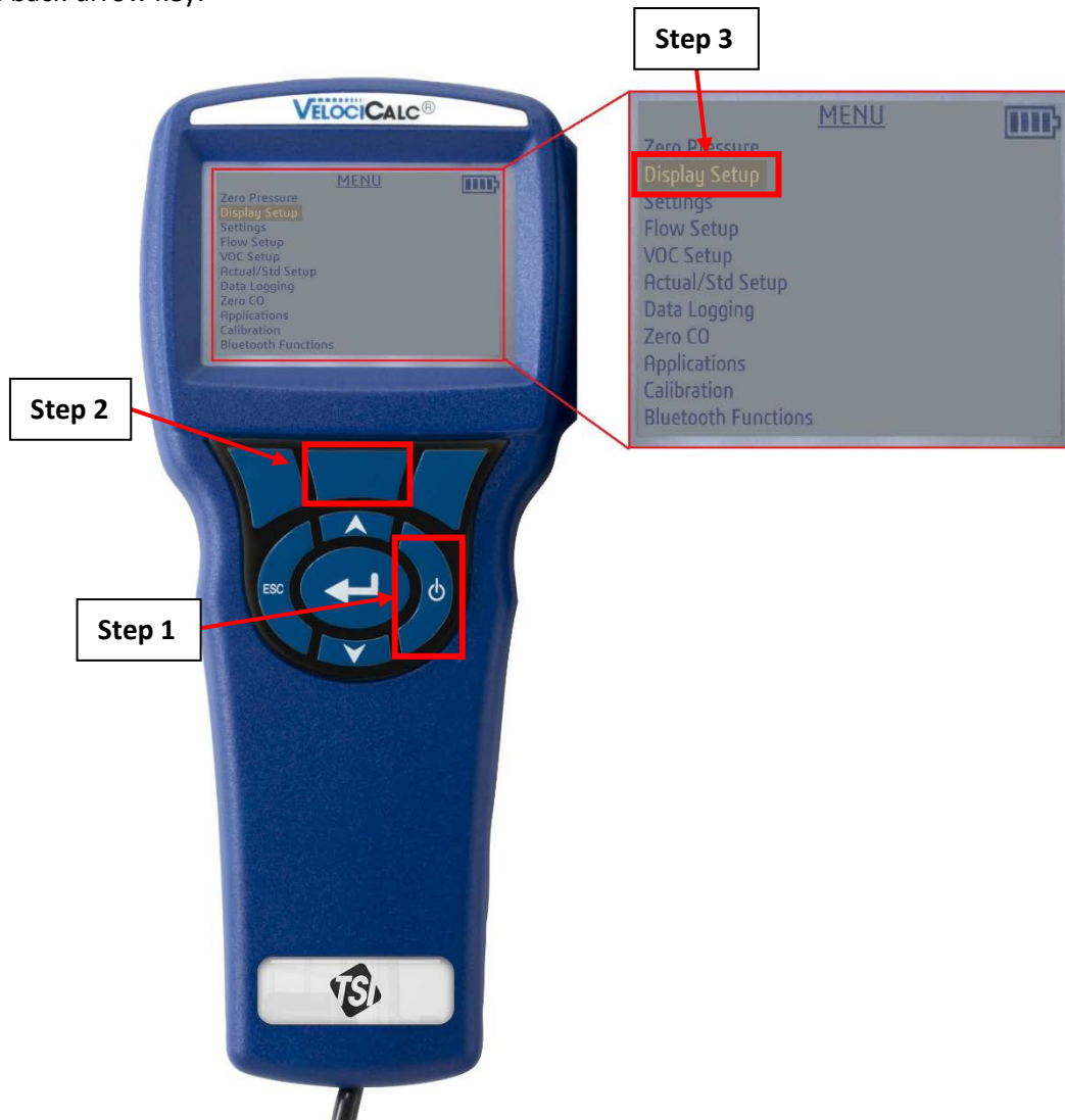
Figure A.10.1: The TSI-9545 Air Velocity Meter's "Menu" screen.
