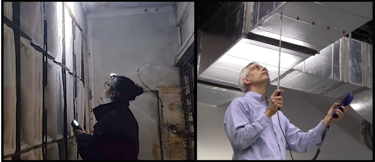
Figure A.10.11: Taking measurements with respect to a ductless airflow is shown on the left. Taking measurements inside a duct is shown on the right.
