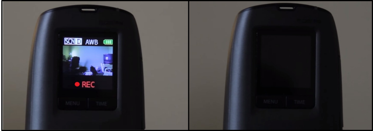
Figure A.11.13: The Brinno TLC200 Pro Time Lapse Camera's recording screen shown on the left. After several seconds, the screen will automatically turn off as shown on the right.
