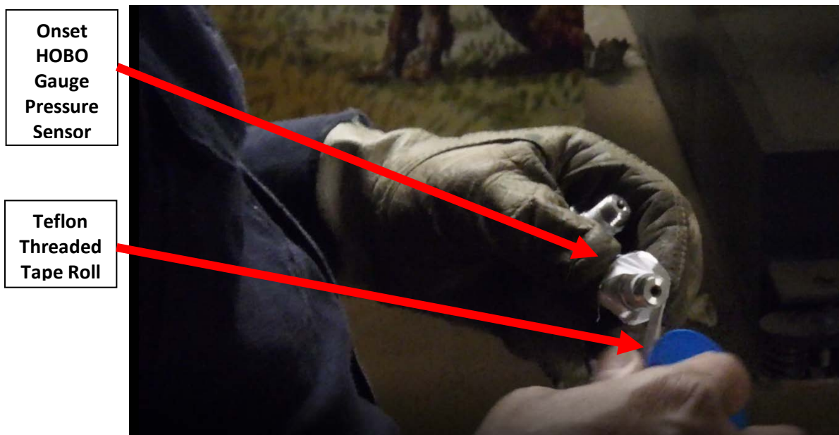
Figure A.9.15: Wrapping Teflon threaded tape around the threads of an Onset HOB0 Gauge Pressure Sensor.
