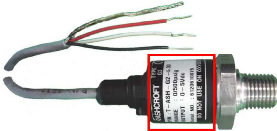
Figure A.9.3: The Onset HOB0 Gauge Pressure Sensor (T-ASH-G2-500).
